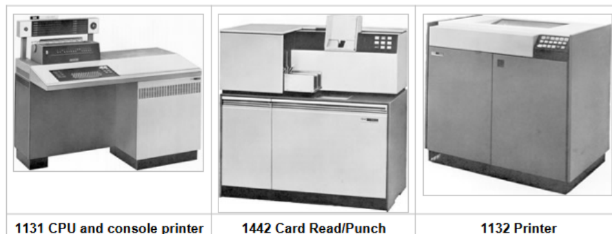
Figure 1: 1130 system: CPU, Card reader/punch, and printer
